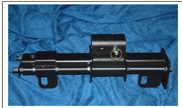
Figure 2. The SFA-16-1100 combined with a Polar Focus Motor Zbeam ® , supporting a JBL Vertec VT4888-AF line array frame. This hardware configuration allows for pan and tilt control of the line array while under load. The line array can also be raised or lowered for service using only one electric chain hoist.
