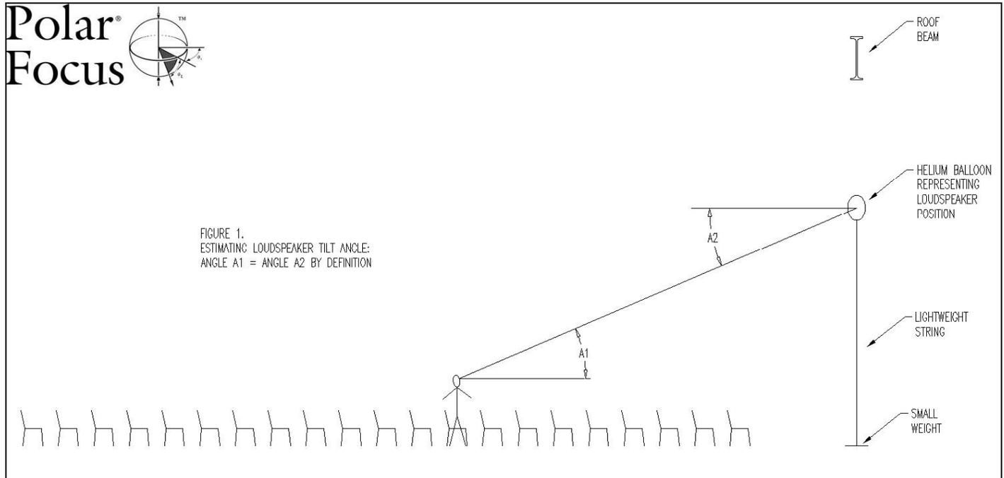
To measure the vertical coverage angle required in an audio installation, you'll need to perform two angular measurements and a subtraction. As shown in Figure 2 below, take an angular measurement
