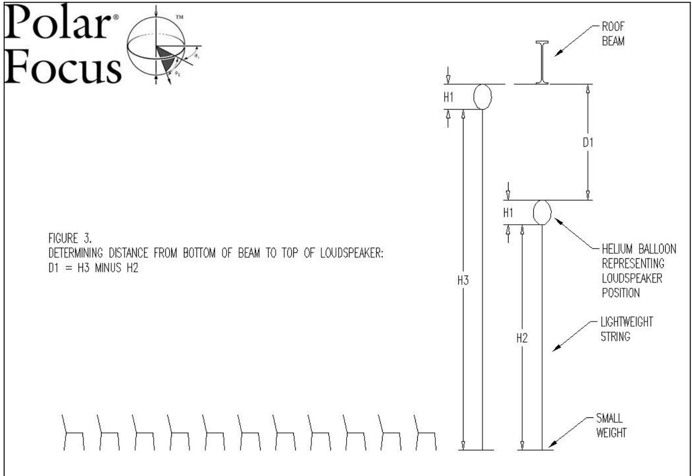
After the loudspeaker position is defined, measure the length of the string H2. Float the balloon up until it just touches the bottom of the beam, then measure the string length H3. Subtract H2 from H3 to determine the distance from the bottom of the beam to the top of the loudspeaker. Adding dimensions H1 and H3 lets you confirm the height of the bottom of the beam above the finished floor.
