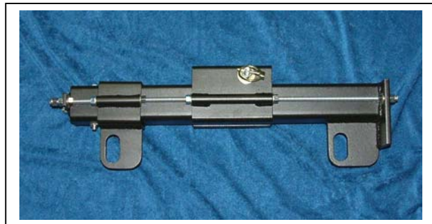
Figure 2. The SFA-16-1100 combined with a Polar Focus Motor Zbeam ® , supporting a JBL Vertec VT4888-AF line array frame. This hardware configuration allows for pan and tilt control of the line array while under load. The line array can also be raised or lowered for service using only one electric chain hoist.
